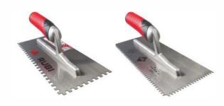
Once your subfloor is clean and dry, spread the adhesive on the surface to be covered with a 10x10mm square toothed trowel, covering an area 5-10cm more than the size of the tile Always apply the adhesive in stripes running parallel with the short edge to remove air pockets and bubbles. By using this method, full coverage of the tile with adhesive is ensured.
